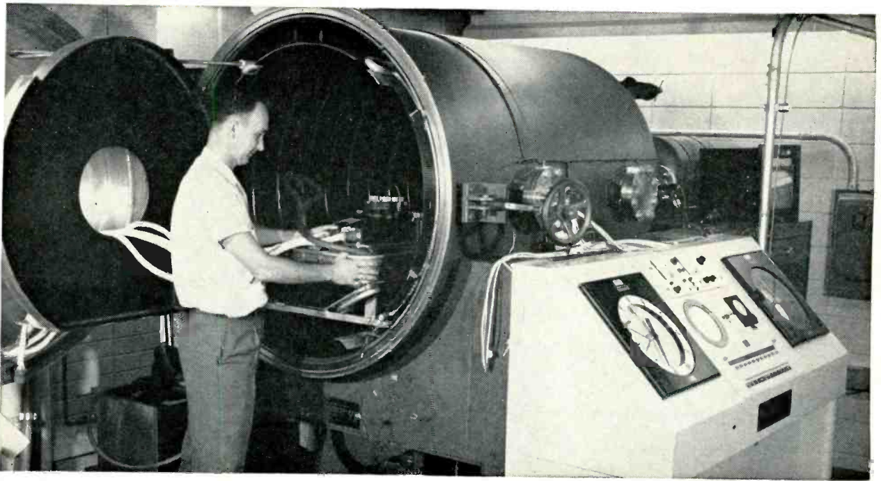
Spaceborne data-transmission equipment is given extensive environmental tests under temperature extremes at low pressure.
