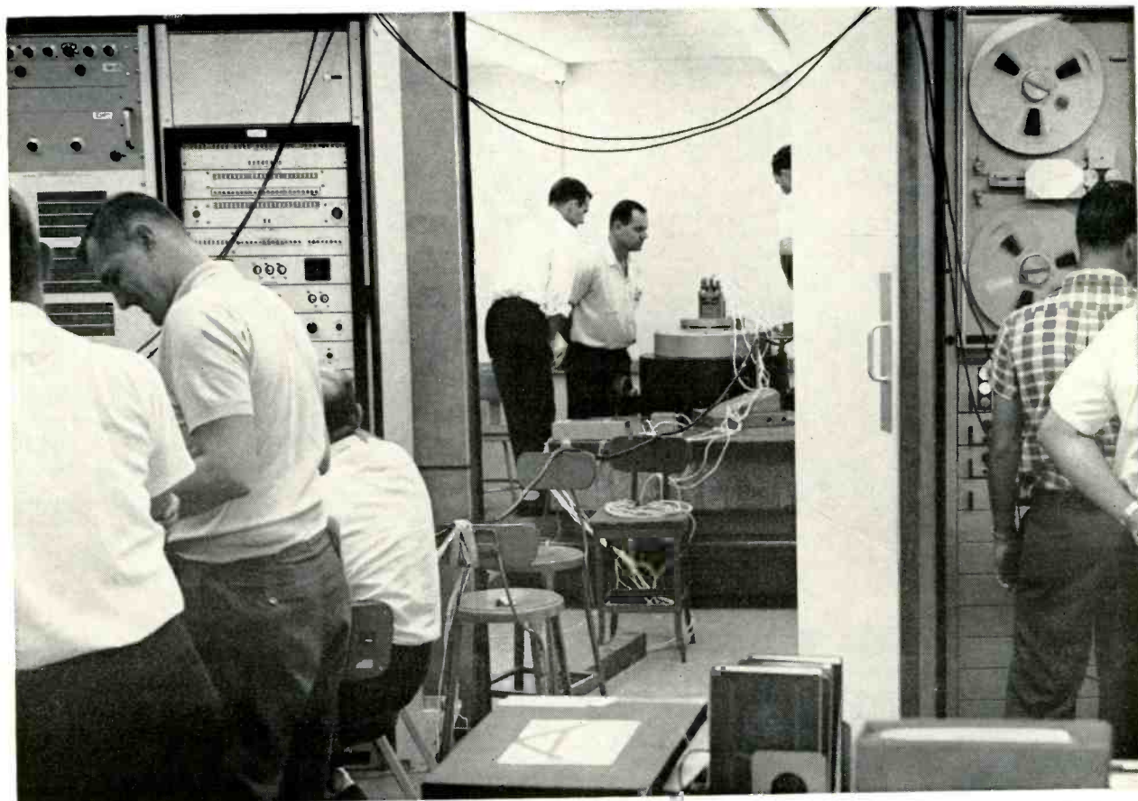
Vibration tests in progress on Gemini equipment (far room) are monitored and recorded for playback and analysis.
