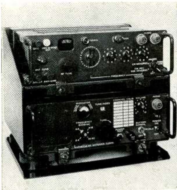
The Army's AN/PRC-62 will be of two types—vehicle (shown above) and man-pack. It will be all transistorized except for the transmitter output stages.
